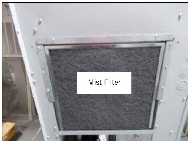
FIGURE 26 Install Mist Filters
